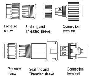
2.Insert the stripped and bared cable through pressure screw, seal ring, threaded sleeve in sequence, insert cables into connection terminal according to polarities indicates on it and tighten the screws firmly. Please try to pull out the wire to make sure the it's well connected.
