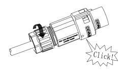
4. Finally, Push or screw the threaded sleeve to connection terminal until both are locked tightly on the inverter.
