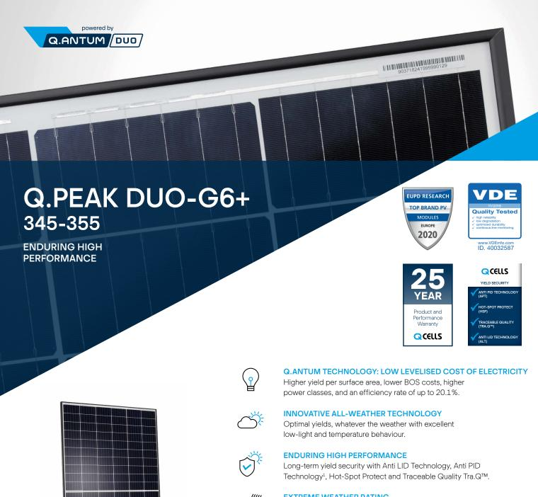
**EXTREME WEATHER RATING**High-tech aluminium alloy frame, certified for high snow (5400 Pa) and wind loads (4000 Pa).
