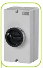
Specifically developed for arduous DC disconnect applications, the IMO range of Solar Isolators features an operator independent trigger ratchet switching mechanism resulting in switching times of less than 5ms. High reliability knife edge contacts and long arc cooling chambers ensure safe and effective isolation of DC voltages within solar installations.
